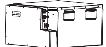
ESTIMATED BATTERY MODULE WEIGHT = 127KG
